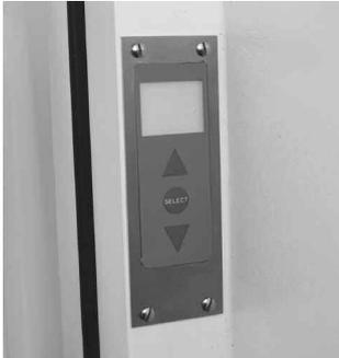
This switch has been designed to fit flush for Installation in hollow Aluminium frame sections and Hollow walls. You will need to cutout/remove part of the Section wall and drill 4 x fixing holes in accordance with the Sizes given in the Instructions supplied with this type of Switch.
