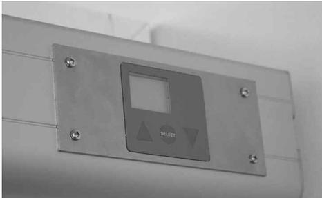
This switch has been designed to fit flush for Installation in the Canopy of the operator. Careful consideration should be paid to the Location of this so it does not affect any internal workings of the operator. You will need to cutout/ remove part of the canopy Section and drill 4 x fixing holes in accordance with the Sizes given in the Instructions supplied with this type of Switch.
